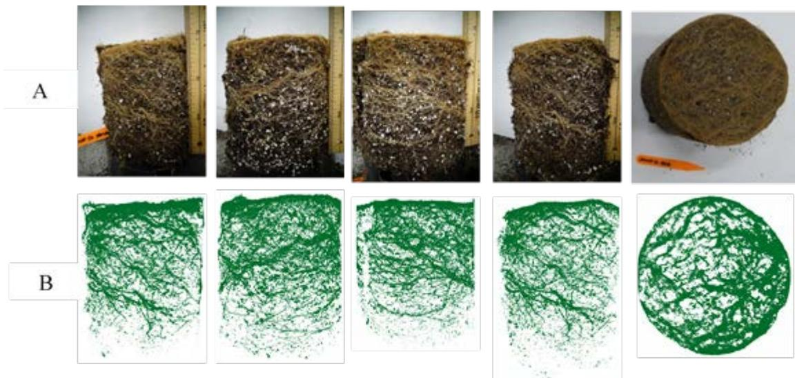
*Figure 1: An example of image classification for root density estimation: (A) original photo, (B) output raster file showing root (green) and background (white).*
