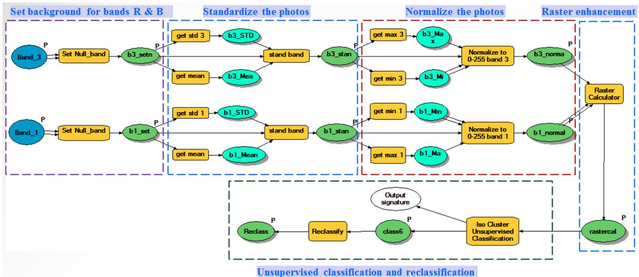
Figure 2: An automated process for data modification using ModelBuilder of ArcMap.
