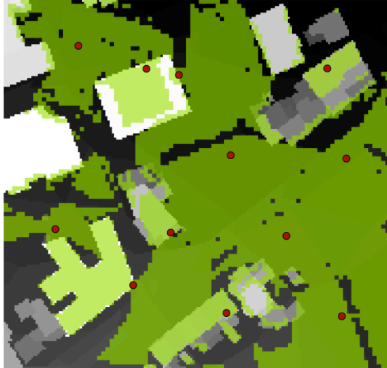
Figure 4: Coverage map of deploying 12 sensors using the context-aware method, considering the terrain model.
