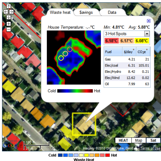
Fig 1: Three circles (inset) automatically define the 3 hottest locations on a home – which in this case fall above 4 sky-lights (inside yellow box). Individual homes (i.e., colored polygons) are designated one of 10 colour classes based on their average roof top temperature .
